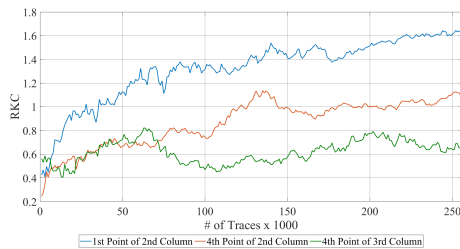
Figure 12. Progressive RKC plot of CPA results for three different situation of horizontal leakage. The red and the green RKC curves relate to when the CUA and the sensor stick to auxiliary circuits, respectively. For the blue one, none of them affected by auxiliary circuits.
