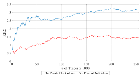
Figure 15. Progressive RKC plot of CPA result for 2 different situation of vertical leakage. The red curve relate to when the CUA and the sensor stick to auxiliary circuits, respectively. For the blue one, none of them affected by auxiliary circuits.
