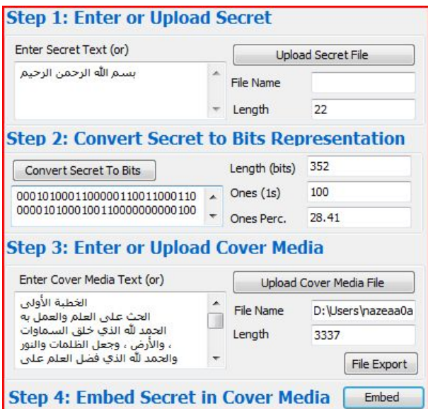
Figure 5. Snapshot of the MSCUKAT program - in focus the steps of encoding a secret
