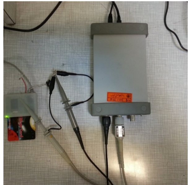
Figure A.1. Experimental setup: data acquisition during encryption
